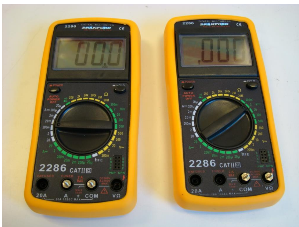
Figure 2.3 Multimeters equipped with terminals for use as ammeter ( left ) and voltmeter ( right ), respectively. The instrument is turned on by pressing “POWER” in the top left corner. The instrument turns off automatically after a certain idle time. It can measure direct current and voltage (=) as well as alternating current and voltage (~). The internal resistance in the voltmeter is 10 M \Omega regardless of the measuring range. The potential difference over the ammeter is 200 mV at full reading, regardless of the measuring range. In case of overflow the display will show “I”, and you need to select a higher measuring range. The “HOLD” button (top right corner) should not be pushed, except if you want to freeze a measurement.
