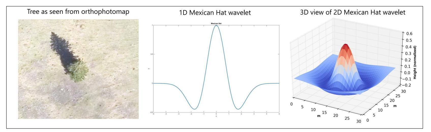
**Study objective:** implement a technique for automatic ecological feature detection (trees and bushes) from a high-resolution LiDAR Canopy Height Model.
